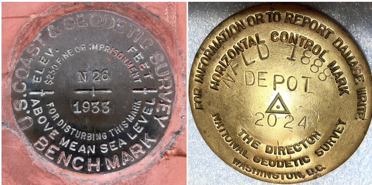
The original geodetic disk (left), used by surveyors, was installed in the depot wall but decommissioned when the depot was moved. The agency gave us a new disk (right) to install on a permanent, horizontal surface open to the sky at the new site.
